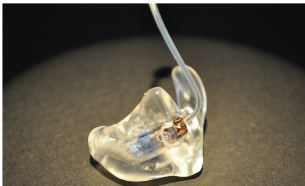
Figure 2. Ear mold with embedded receiver
